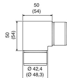
Rohrverbinder | tube connector
