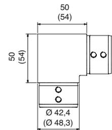
Rohrverbinder | tube connector
