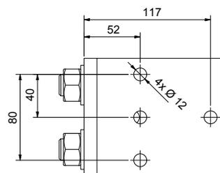
Anzugsmoment | tightening torque M20: 322Nm + 60°
